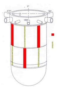
The target flaw size for the inspection was 10mm x 10mm quasi lamination defects, oriented parallel to the inner and outer surfaces of the RPV. The inspection results showed that no unacceptable defects have been detected within the inspection volumes of any of the six segments of base material. Besides, only three reportable indications have been detected in the lower shell:
