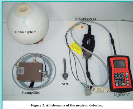
Figure 3. All elements of the neutron detector.
