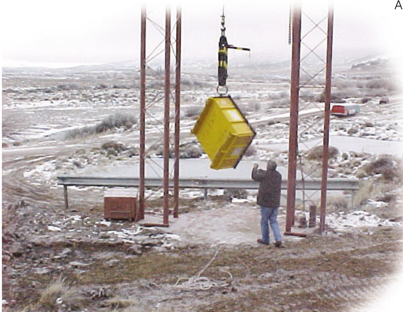
Accidental conditions of transport: mechanical test
