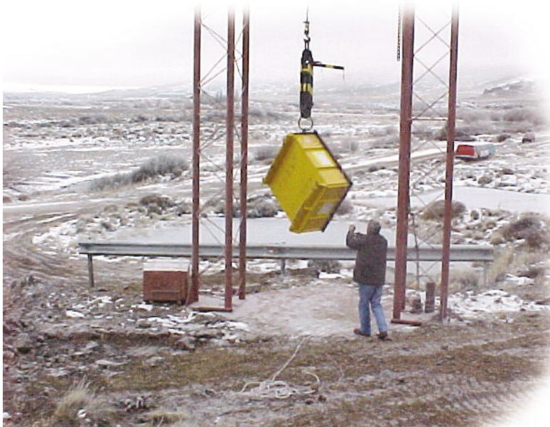
Accidental conditions of transport: mechanical test
