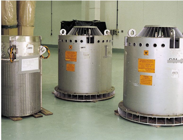
Type B (U) packages for cobalt 60 transport. GURI 01 (centre and right) and F129 (left) models.
